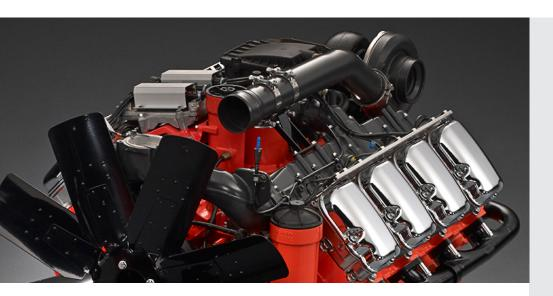
The engines for power generation from Scania are based on a robust design with a strength optimised cylinder block containing wet cylinder liners that can easily be exchanged. Individual cylinder heads with 4 valves per cylinder promotes repairability and fuel economy.
